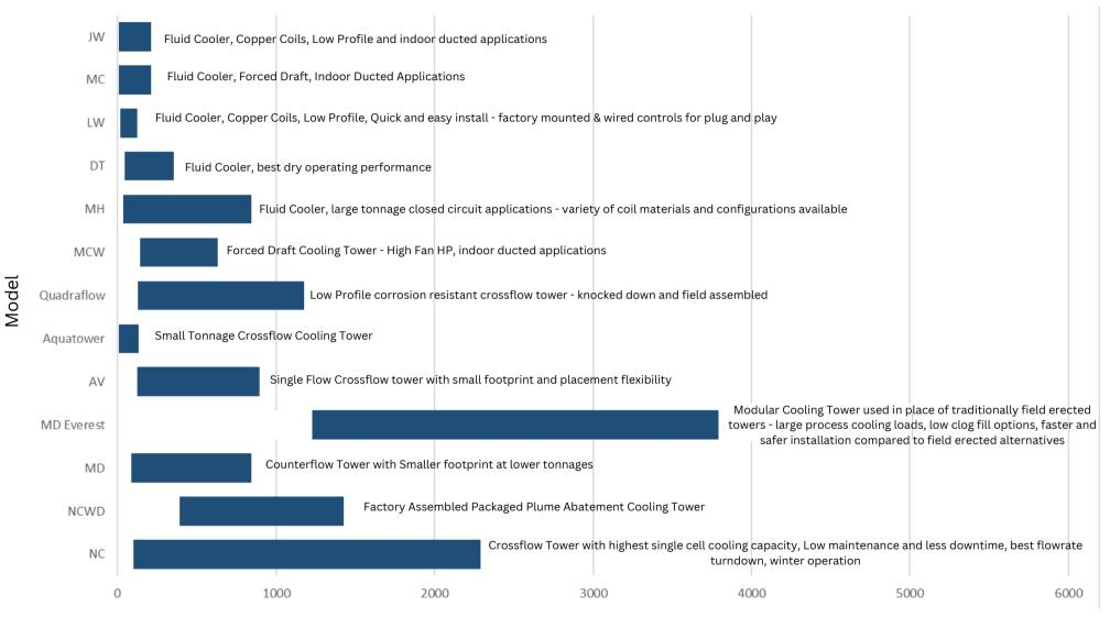
Thermal Capacity (Nominal Tons/cell\*)
